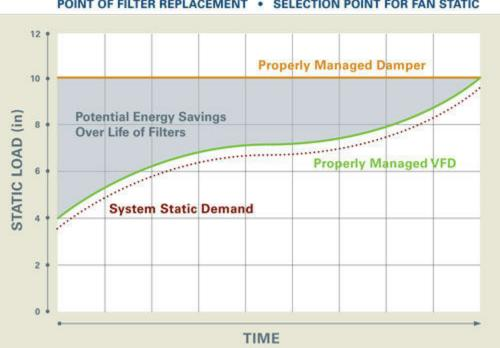
POINT OF FILTER REPLACEMENT . SELECTION POINT FOR FAN STATIC
